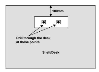
**3.** From underneath the desk, push two bolts through the base plate and secure to the internal anchor plate. Place the nuts on the bolts and tighten using the supplied spanner.
